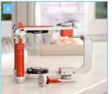
Remove the anterior guide pin incl. holder and place the anterior guide table into the top half of the articulator. Insert the **CORSOFIX®** transfer jig as far as it will go in the bottom half of the articulator and screw to secure. Now place the anterior guide table in the top half of the articulator, with the smooth side on the **CORSOFIX®** transfer jig support.
