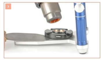
Using a hot air gun, apply heat uniformly to the centre of the **ADESSOSPLIT®** calibration base plate. After approx. 30–60 seconds, use a wax or plaster knife to release the plate from the bottom half of the articulator. Caution: Risk of burn injury – always work on a heat-resistant surface!
