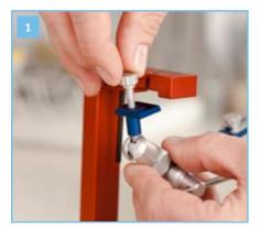
Insert the CORSOFIX® joint support into the socket provided in the ADESSOSPLIT® transfer stand.
