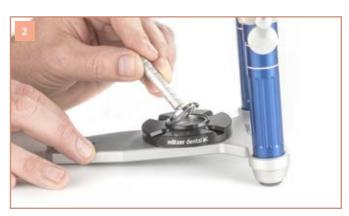
Use a magnet pickup tool to lift the magnets out sideways.
