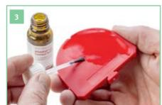
Using the brush, apply the **DIVARIO® 3D primer** (art. no. 14601) evenly to the entire surface of the **DIVARIO® base plate** and leave to air-dry for approx. 1 minute.
