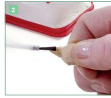
The **die protector** soaks into the porous surface of the die and protects it from material abrasion. This works to reduce reflections while fixing markings in place.
