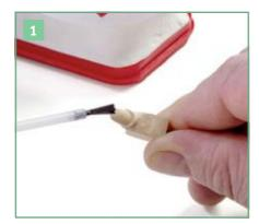
The first coat of **die protector** is applied to the stone die.
