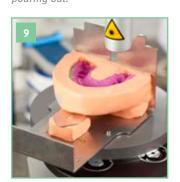
Place the **DIVARIO®** impression carrier L with the DIVARIO® Duo plate support onto the magnetic plate on the **DIVARIO® M23** compact pin drilling unit.
