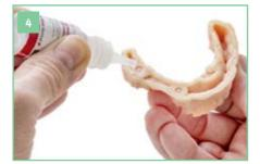
Apply a sufficient quantity of **DIVARIO® 3D** model glue (art. no. 14602) evenly to the underside of the 3D printed model, so as to fill any gaps between the 3D model and the base plate.
