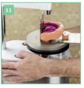
Press the button to start drilling - the **DIVARIO® Duo plate support** is held in place electromagnetically.
