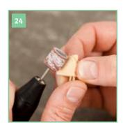
Work the individual segments with a **DIVARIO®** finishing strip and clean to remove die stone dust.
