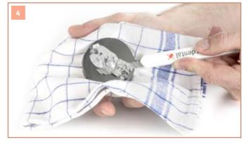
Any residues of metal adhesive can be removed from the **ADESSOSPLIT®** calibration base plate using a utility knife re-heat the ADESSOSPLIT® calibration base plate with the hot air gun if necessary. Caution: Risk of burn injury – use safety gloves or a heat-proof cloth!
