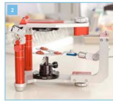
Place the CORSOFIX® bite fork support in the centre of the ADESSOSPLIT® calibration base plate. Fix the CORSOFIX® joint support to the CORSOFIX® transfer jig.
