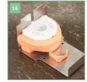
Once pinned, check the **DIVARIO**® base plate by placing it in the impression.
