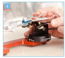
Move the ADESSOSPLIT® transfer stand into position. The distance between the CORSOFIX® bite fork and the retention screws should be approx. 5 mm. The height of the ADESSOSPLIT® transfer stand can be adjusted by undoing the socket head screw.
