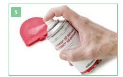
Next, spray **DIVARIO® 3D activator** (art. no. 14603) from a distance of about 30 cm to create a thin, even coat on the **DIVARIO® base plate**. Leave to air-dry for about 30 seconds until the surface turns matt.
