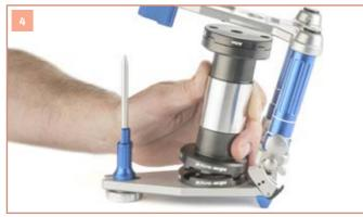
Close the **CORSOART®** articulator before applying adhesive. Ensure a bond line of 1-2 mm between the ADESSOSPLIT® calibration base plate and the articulator bottom half; ensure the incisal pin is in contact with the anterior guide table.
