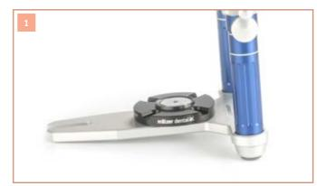
To release the ADESSOSPLIT® calibration base plate, remove the top half of the articulator and the anterior guide table.
