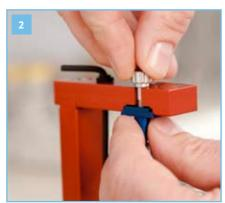
Hold the grooved pin from the CORSOFIX® joint support in place in the ADESSOSPLIT® transfer stand and secure with the screw.
