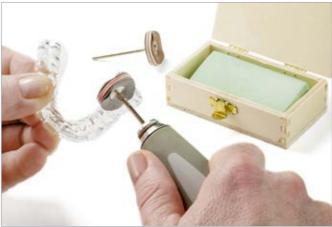
Pre-polish and final polish of a PMMA night guard, with the Alcontura soft microfibre buff disk.
