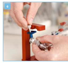
Place the CORSOFIX® joint support at a slight angle in the socket provider on the ADESSO-SPLIT® transfer stand and lay the CORSOFIX® bite fork into the mixed plaster.
