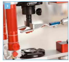
Turn the **CORSOART®** articulator upside down and let the crossbar on the **CORSOFIX®** bite fork support fall onto the CORSOFIX® bite fork. Fix the CORSOFIX® bite fork support in place by tightening the knurled screw.
