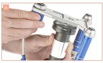
Tilt the **ADESSOSPLIT®** centring key backwards slightly in order to close the CORSOART® articulator.Let the ADESSOSPLIT® metal adhesive cure for approx. 160 min. with the CORSOART® articulator closed. Use a rubber band to fix the CORSOART® articulator in place. Make sure that the incisal pin is supported by the anterior guide table.
