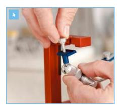
Once positioning is correct, remove the CORSOFIX® joint support from the ADESSOSPLIT® transfer stand.
