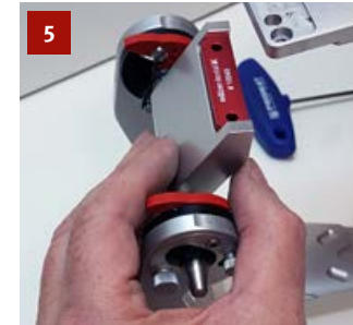
Place the red block of the extension set on the articulator – text side up.
