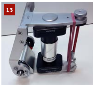
Fix the articulator in place using a rubber band and let the adhesive cure for approx. 90 min.
