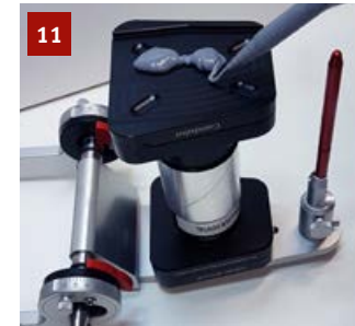
Invert the centring key together with the calibration base plate in the articulator and apply metal glue to the center of the plate.
