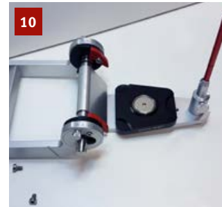
The base plate will be fixed in the upper part of the Candulor® plate magnetically, supported by the metal glue.
