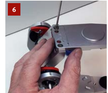
Fix the upper part of the articulator with the new, longer screws.
