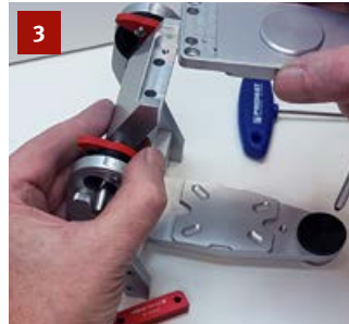
Loosen two screws and lift the upper part of the articulator. Attention: Do not use the screws again.
