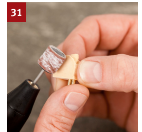
Work the individual segments with a DIVARIO® finishing strip and clean to remove plaster dust.
