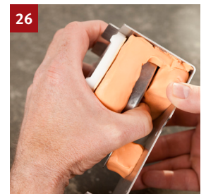
After approx. 25 minutes, carefully remove the impression together with the DIVARIO® base plate .
