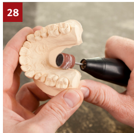
An alternative to a model trimmer, work the dental model freehand with a DIVARIO® finishing strip .
